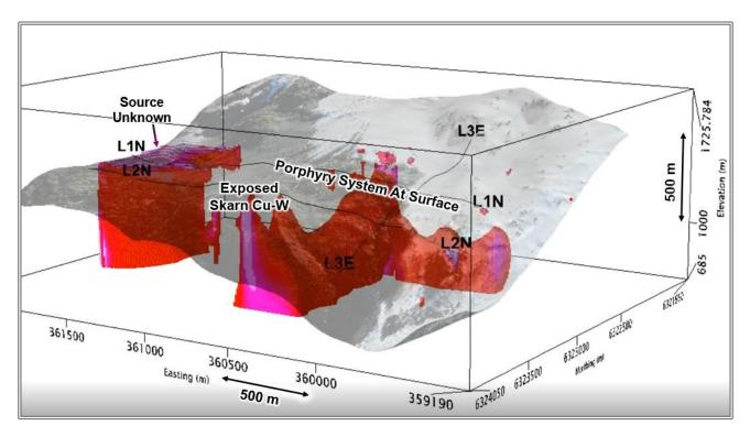
Figure 1: Southeast looking orthogonal view of the Trek South 3D chargeability model derived from IP data. Chargeability highs in red are believed to reflect sulphide mineralization beneath the exposed porphyry and skarn mineralization.
